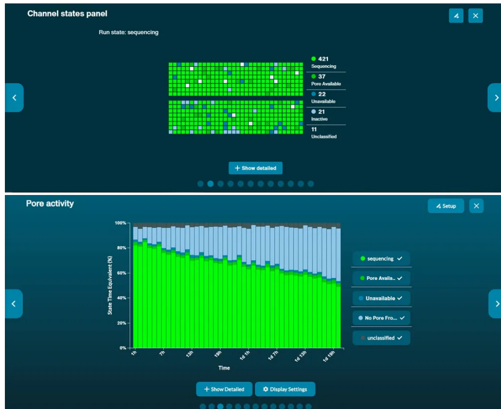
Figure 5. Light green: sequencing, Dark green: open pore, Dark blue: pore recovering, Light blue: pore inactive.
